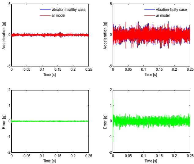
Figure 6. Original vibration signals and their predictions using  $AR$  method for healthy and faulty cases of motor (upper plots), and the residuals computed as the difference between them (lower plots).
