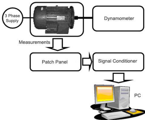
Figure 2. Motor load testing and data acquisition system.
