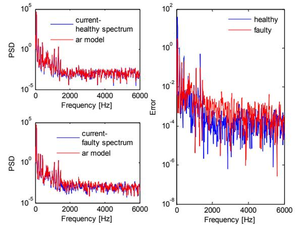
Figure 7.  $PSDs$  of original current signals and  $PSDs$  of their predictions using  $AR$  method for healthy and faulty cases of motor (left plots), and the error computed as the difference between them (right plot).
