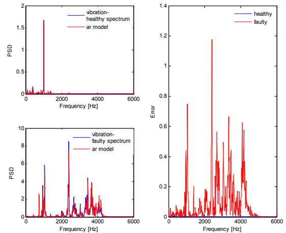
Figure 8.  $PSDs$  of original vibration signals and  $PSDs$  of their predictions using  $AR$  method for healthy and faulty cases of motor (left plots), and the error computed as the difference between them (right plot).
