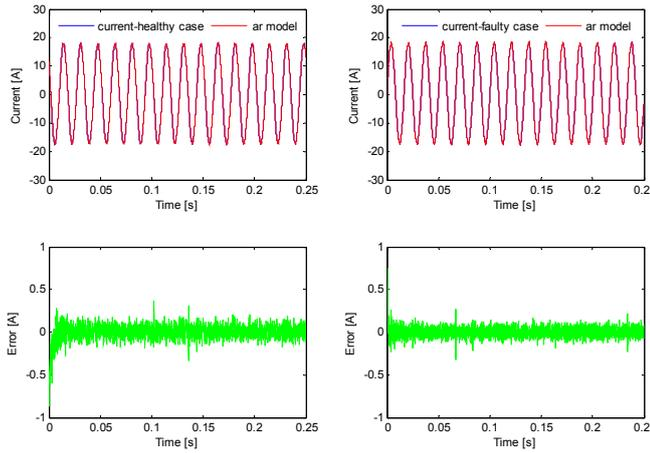
Figure 5. Original current signals and their predictions using  $AR$  method for healthy and faulty cases of motor (upper plots), and the residuals computed as the difference between them (lower plots).
