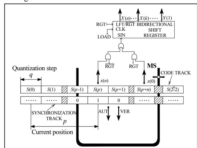
Figure 1. Serial pseudorandom code reading with two reading heads
