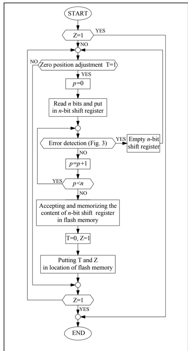
Figure 4. Direct zero position determination method
