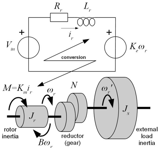
Figure 2. Basic electro-mechanical model of a typical R/C servo.
