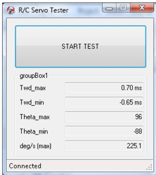
Figure 7. Screen-capture of the control application showing the test results
