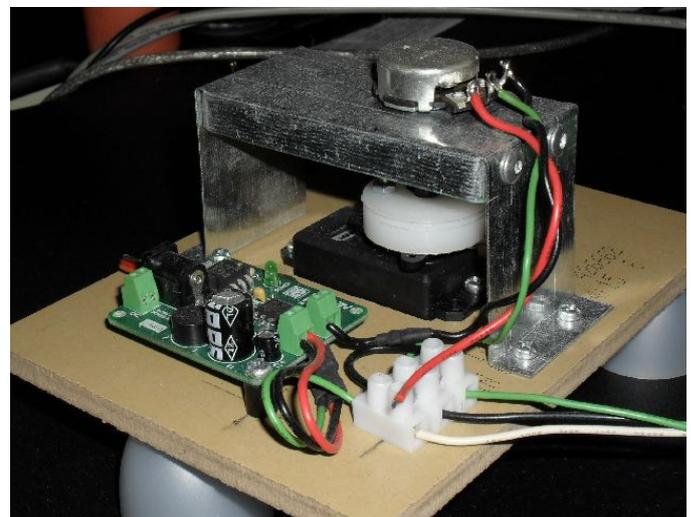
Figure 6. Photograph of the mechanical parts of the R/C servo testing platform. The power source, the feedback potentiometer and the R/C servo itself connected to it via a plastic disc can be seen in the picture.
