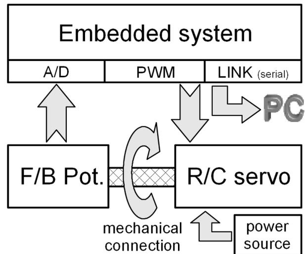
Figure 5. Block diagram of the automated R/C servo testing platform
