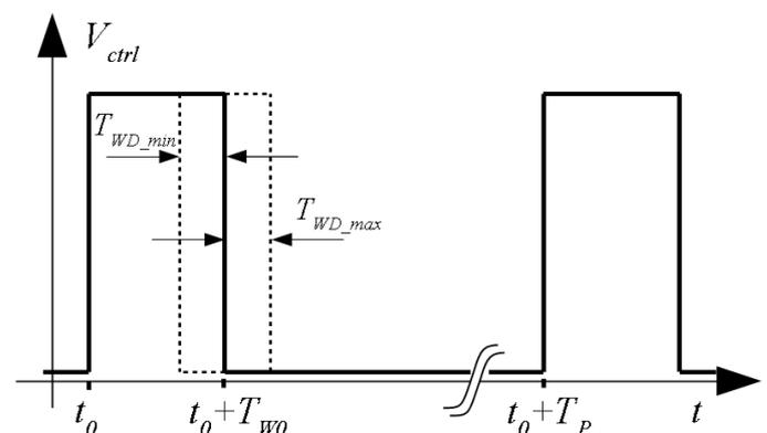
Figure 1. Explanation of the pulses required to command a typical R/C servo to the required angular position
