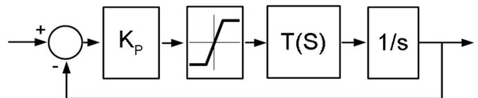
Figure 3. Diagram of the servo control loop
