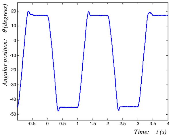
Figure 4. Typical response of an R/C servo to a step-input of a sufficiently large amplitude – captured by a Picoscope 3000 USB oscilloscope. The change of the angular position in time is presented here. The linear, constant-slope parts indicate that the DC motor's velocity limit has been reached during each transition
