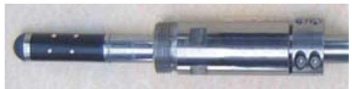
Figure 3. Two-component electromagnetic probe [1]
