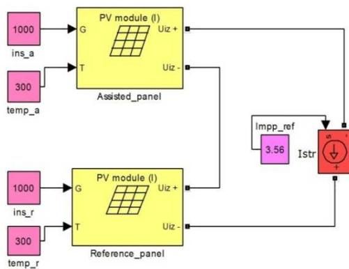
Figure 6. Simulation scheme without power optimizer
