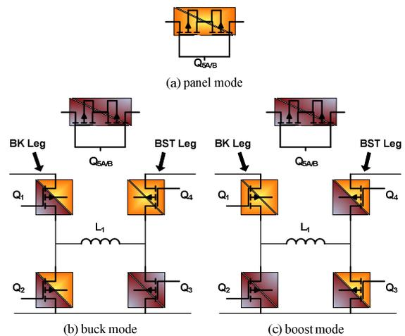
Figure 4. Operating modes of buck-boost converter
