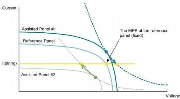
Figure 2. I-V curve of a single string with partial DC-DC units (1 reference panel and two assisted panels)
