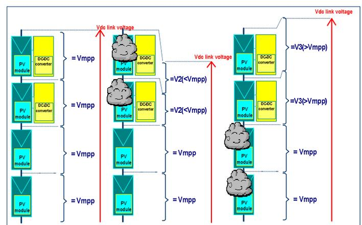
Figure 1. Buck and boost operating modes of DC-DC converters
