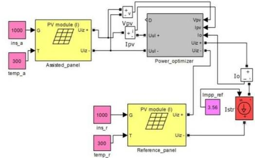
Figure 5. Simulation scheme with power optimizer
