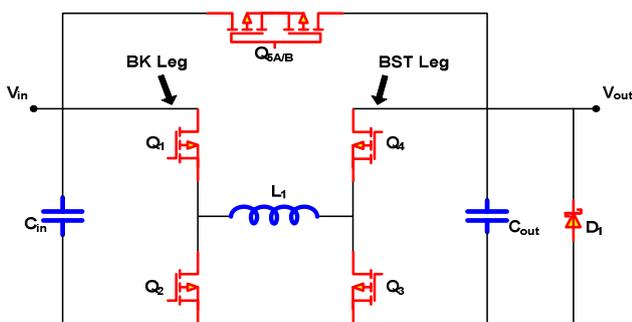
Figure 3. Selected topology of synchronous rectifier
