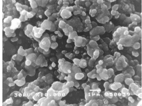
Figure 6. SEM image of 0.5 mol% Nb/BaTiO<sub>3</sub> sintered at 1320°C
