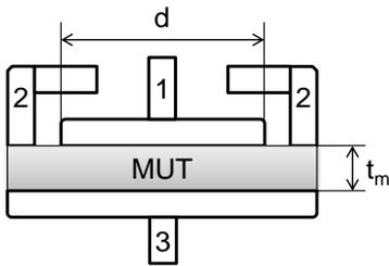
Figure 2. Illustration of contacting electrode method (1 – guarded electrode, 2 – guard electrode, 3 – unguarded electrode)
