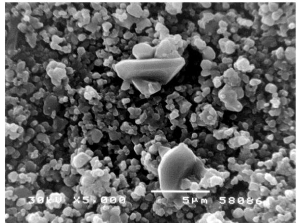
Figure 7. SEM image of 2 mol% Nb/BaTiO<sub>3</sub> sintered at 1320°C
