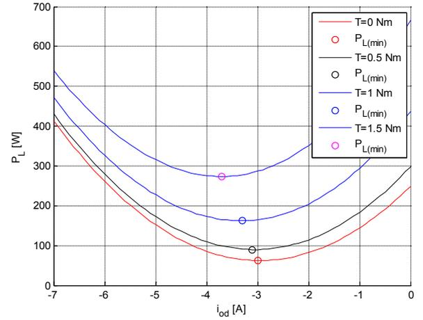
Figure 5. Electrical losses as function of  $i_{od}$  and T at 14000rpm
