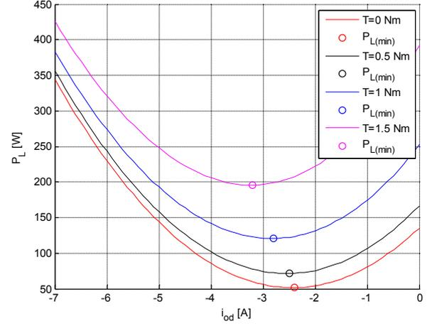
Figure 4. Electrical losses as function of  $i_{od}$  and T at 7000rpm
