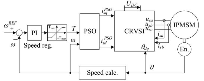
Figure 3. PSO based energy efficient IPMSM drive
