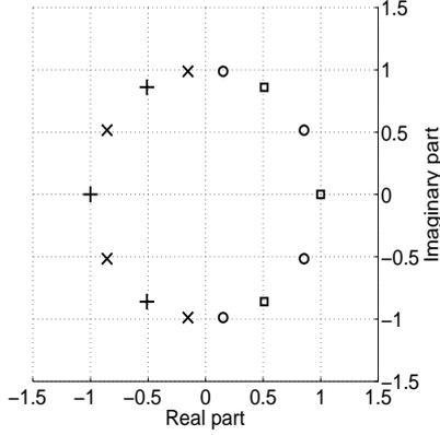
Fig. 3. Pole-zero plot of allpass functions in  $s$ -plane of the 7th-order prototype for transfer function with  $R_s = 40$  dB,  $M = 1$  and  $l_1 = 1$ . Poles and zeros of  $A_1(s)$  are tagged with  $\times$  and  $\circ$  respectively; but poles and zeros of  $A_2(s)$  are tagged with  $+$  and  $\square$  respectively.
