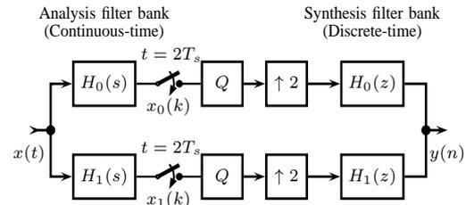
Fig. 1. Two channel hybrid continuous/discrete filter bank.
