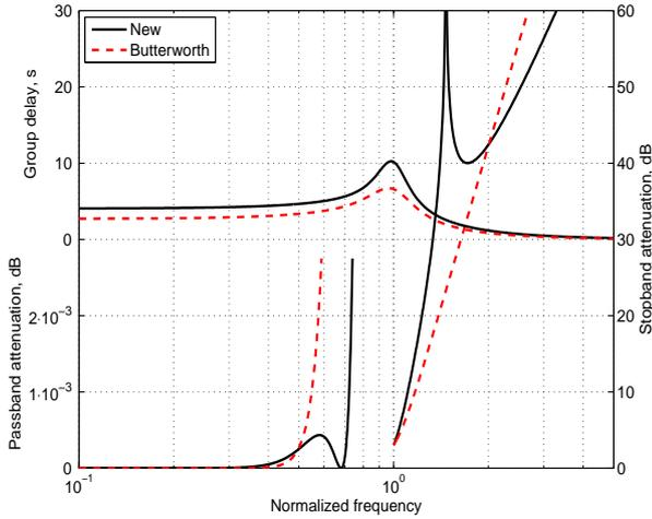
Fig. 4. Comparison of 7th degree new filter frequency responses ( $R_s = 40$  dB and  $k = 5$ ) with 7th degree Butterworth filter frequency responses.
