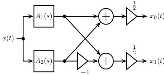
Fig. 2. The system of two-channel power complementary filter bank.
