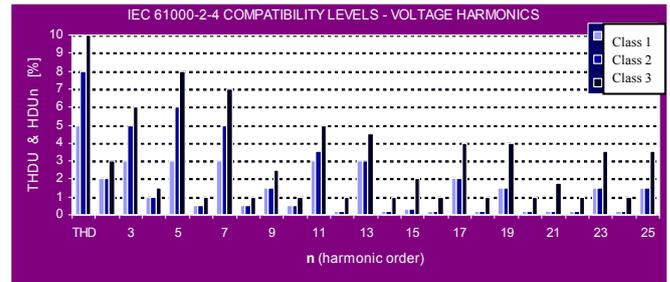
Figure 10. IEC 61000-2-4 Compatibility levels for MV voltage harmonics [19]
