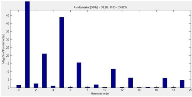
Figure 6. Phase current harmonic spectrum at the charging station input terminals (Mode 3).
