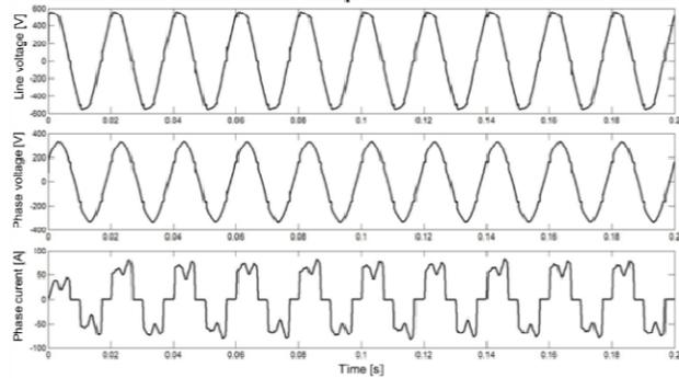
Figure 7. Line, phase voltage and phase current at the charging station input terminals (Mode 4).
