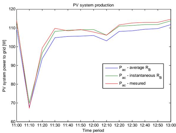
Figure 7. Experimental results of PV system output power compared with estimating ones based on different calculation way of slope factor.
