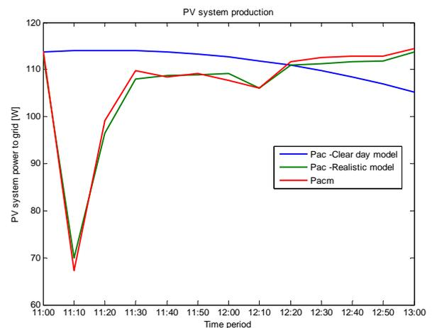
Figure 5. Experimental results of PV system output power with estimating one obtained with given models.
