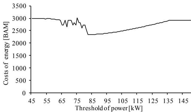
Figure 5. Cost of energy in function of power threshold
