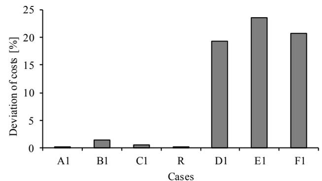
Figure 8. Deviation of energy cost from the minimum value
